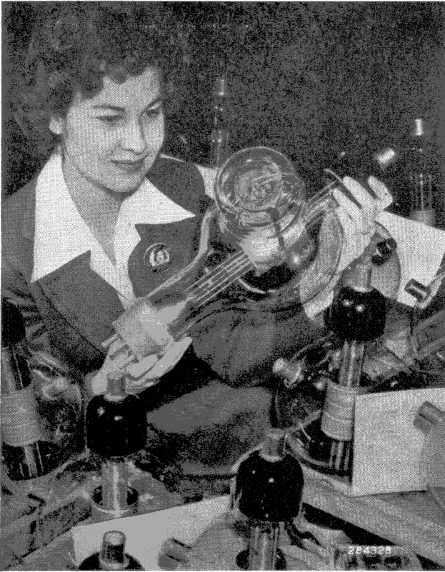
Huge transmitting tubes for the U. S. Navy represent one of the many types of electronic devices required by modern warfare. These tubes make possible fast radio communication between ships at sea and shore stations.
